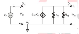
$$\frac{V_{out}}{V_{in}} = \frac{-g_{m2}V_{gs}\left(r_{o2} \mid\mid R_{eq}\right)}{V_{gs}}$$
