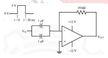
The output voltage VOUT of this circuit at  $t = 0^+$  (in integer) is \_\_\_\_\_V.
