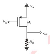
Replace M<sub>2</sub> with small signal model.
