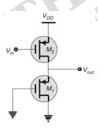
Drain to gate connected MOSFET M<sub>1</sub> acts as load.
