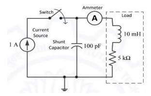
Initially, when the switch is open, the capacitor is discharged and the ammeter reads zero ampere. After the switch is closed, the ammeter reading keeps fluctuating for some time till it settles to a final steady value. The maximum ammeter reading that one will observe after the switch is closed (rounded SU Coaching Institute Since 1997 off to two decimal places) is \_
