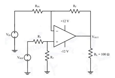
If  $V_{OUT} = 1$  volt for  $V_{IN} = 0$ . 1 volt and  $V_{OUT} = 6$  volt for  $V_{IN} = 1$  volt, where  $V_{OUT}$  is measured across R<sub>L</sub> connected at the output of this OPAMP, the value of R<sub>F</sub>/R<sub>IN</sub> is oaching institute since 1991
