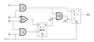
: Maximum propagation delay for the circuit is 6ns.
