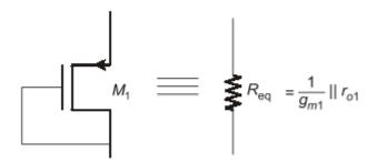
For given circuit, AC equivalent is as shown.
