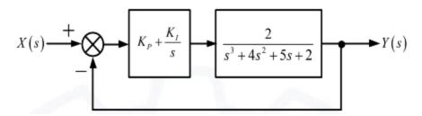
The stability of the overall system is controlled by tuning the PI control parameters K<sub>P</sub> and K<sub>I</sub>. The maximum value of K<sub>1</sub> that can be chosen so as to keep the overall system stable or, in the worst case, coaching institute since 1991 marginally stable (rounded off to three decimal places) is
