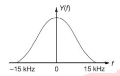
$$NR = 2 \times f_{max} = 2 \times 15 = 30 \text{ kHz}$$
