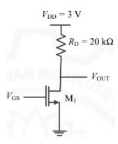
The channel length modulation coefficient is ignored. If the gate-to-source voltage V<sub>GS</sub> is 1 V to keep the transistor at the edge of saturation, then the threshold voltage of the transistor (rounded off to one decimal place) is \_\_\_\_\_\_ V.
