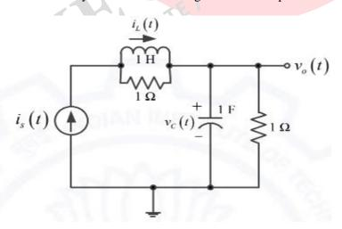
Current  $i_L(t)$  in the inductor and voltage  $v_C(t)$  across the capacitor are taken as the state variables, both assumed to be initially equal to zero, i.e.,  $i_L(0)$  and  $v_C(0) = 0$ . The system is
