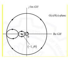
If G(s)H(s) has one zero in the right-half of the s-plane, the number of poles that the closed-loop system will have in the right-half of the s-plane is
