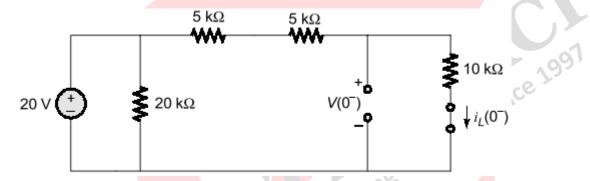
$$i_L(0^-) = \frac{20}{5k\Omega + 5k\Omega + 10k\Omega} = 1 \,\mathrm{mA}$$
