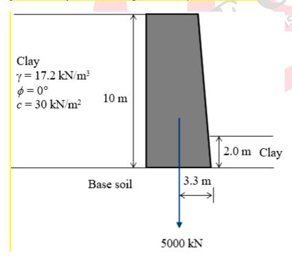
The factor of safety (round off to two decimal places) against sliding failure of the retaining wall after ignoring the passive earth pressure will be \_\_\_\_\_\_.
