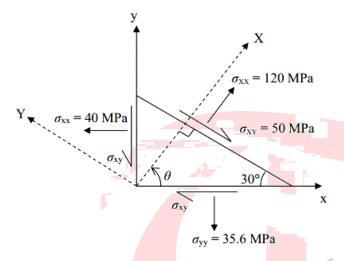
The absolute magnitude of the shear stress components  $\sigma_{xy}$  (in MPa, round off to one decimal place) in x-y coordinate system is U Coaching
