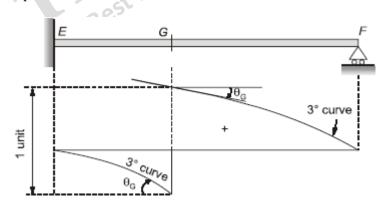
As per Muller Breslau principle ILD for stress function (shear -  $V_G$ ) will be a combination of curves (3° curves).
