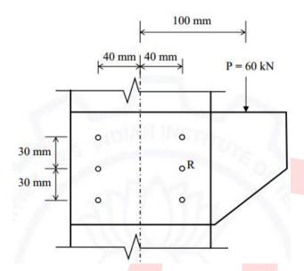
The resultant force in **bolt R** (in kN, round off to one decimal place) is \_\_\_\_\_\_
