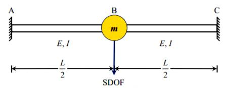
If the flexural stiffness of the beam is  $4\pi^2$  kN/m, its natural frequency of vibration (in Hz, in integer) in the flexural mode will be \_\_\_\_\_.
