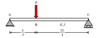
The plastic moment, Mp calculated for the collapse mechanism using static method and kinematic method is
