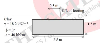
Using Meyerhoff's method, the load (in kN, round off to two decimal places) that can be applied on the footing with a factor of safety of 2.5 is \_\_\_\_\_\_.
