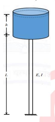
If elastic modulus (E) of steel is 200 GPa, ignoring sel-weight of the tank, for the supporting steel column to remain unbuckled, the maximum depth (h) of the water permissible (in m, round off to one decimal place) is \_\_\_\_\_.
