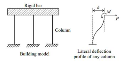
For the lateral deflection profile of the columns as shown in the figure, the natural frequency of the system for horizontal oscillation is
