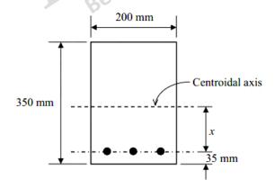
The distance of the centroidal axis from the centreline of the reinforcement (x) for the uncracked section (in mm, round off to one decimal place) is \_\_\_\_\_\_.
