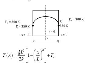
For maximum temperature,  $\frac{dT_x}{dx} = 0 = \frac{\dot{g}L^2}{2k} \cdot \left(\frac{-2x}{L^2}\right)$
