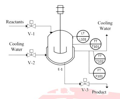
Which one of the following schemes can be used for feedback control? te since 199
