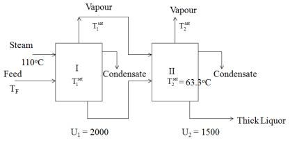
The driving force in evaporators  $\Delta T = T^{steam} - T^{sat}$ As given heat load is same in both effects, i.e.,  $Q_1 = Q_2$ As  $A_1 = A_2$  rule of thumb
